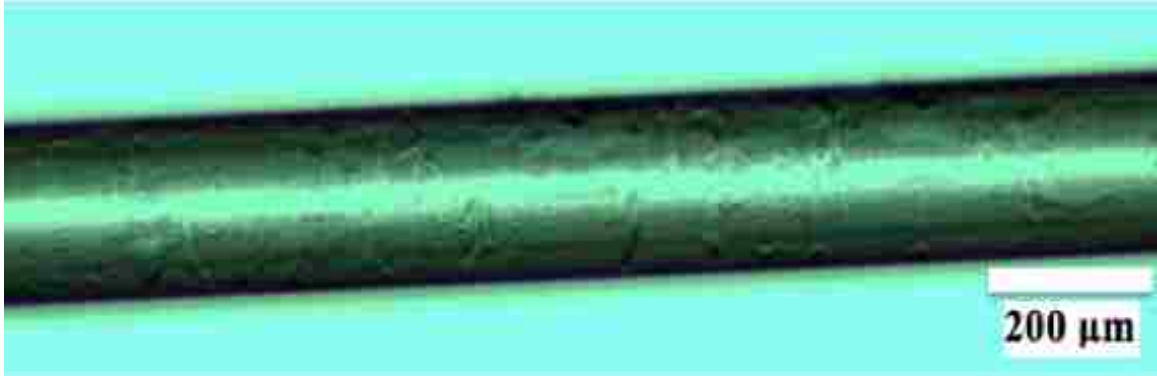
Figure 5.12: Micrograph of a ZBLAN fiber processed at 360°C for 8 minutes.
