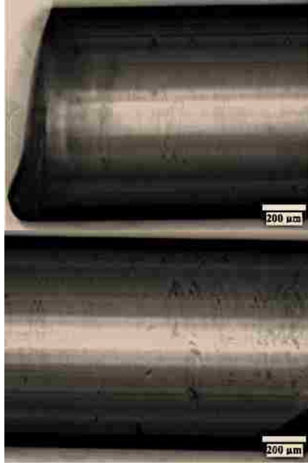
Figure 4.15: Hyper-g ZBLAN sample (top) and 1-g ZBLAN sample (bottom) at 290°C.
