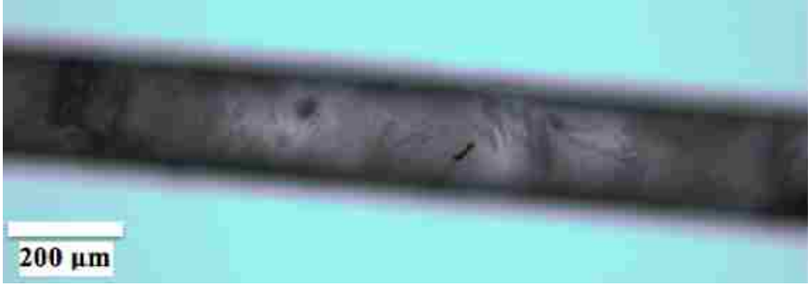
Figure 5.15: Micrograph of a ZBLAN fiber processed at 400°C for 30 seconds.
